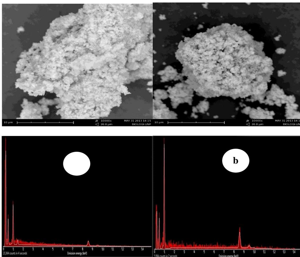
Figure 5: SEM-EDX results of sample ZnO / chitosan a. ZnO-chitosan, b. ZnO-CTAB15%-chitosan30%.
