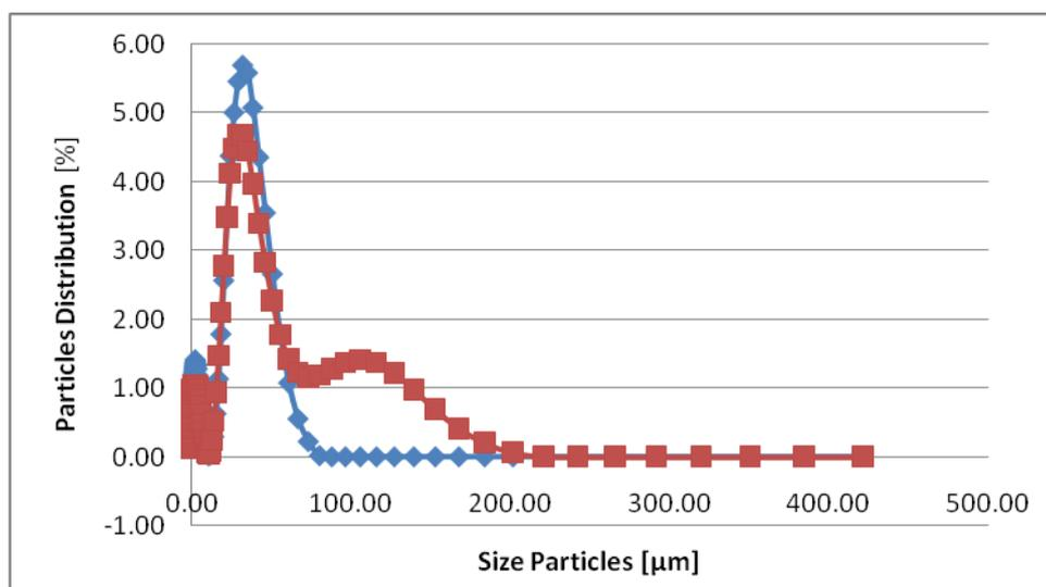
Figure 6: PSA patterns of ZnO samples / Chitosan a. ZnO-chitosan (blue), b. ZnO-CTAB15%-kitosan30% (red)
