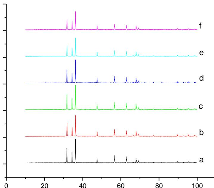
**Figure 4: XRD spectrum with the variation of chitosan. (a) ZnO (b) ZnO-chitosan, (c) ZnO-CTAB, (d) ZnO-CTAB 15%-Chitosan 20%, (e)ZnO-CTAB 15%-chitosan 25%, f) ZnO-CTAB 15% –Chitosan 30%**
