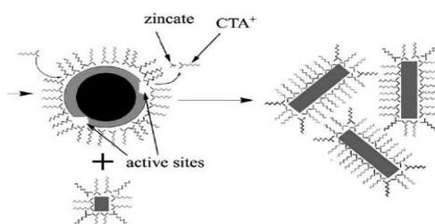
Figure 3: Illustration of ZnO bond with CTAB surfactant
